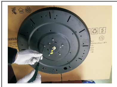
Step 2. Remove the main engine chassis screws.
