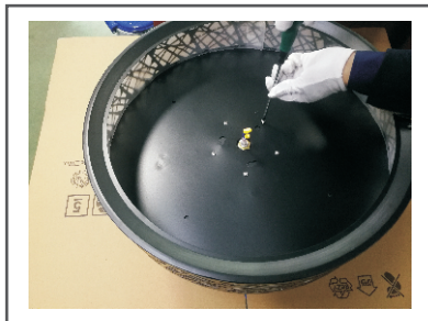
Step 3. Install and fix the lampshade on the chassis with screws.
