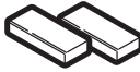
Filler blocks or scrap wood pieces (for top cabinet spacing in recessed bottom cabinet installations, if needed)
