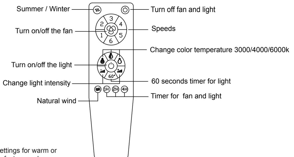
The appropriate speed settings for warm or cool weather depends on factors such as the room size, ceiling height and number of fans.
