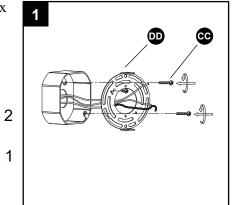
2. Strip 3/4 in. of insulation from wire ends. Twist stripped ends together with pliers (not included), black to black (power) and white to white (neutral). Attach copper wire to ground wire. Helpful hint: If necessary, attach copper ground wire to grounded outlet box.
