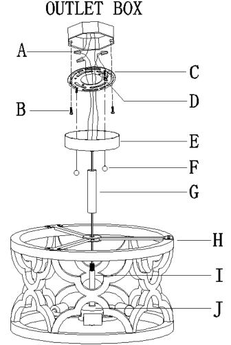
2. Unscrew knob nuts (F) from canopy (E), then gently remove mounting plate (C) from canopy (E) and set them aside for later installation.
