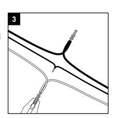
4. Attach wire nuts (BB). Tape wire nuts (BB) and wires together.
