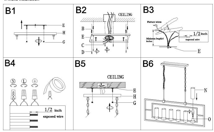
Step B1: Unscrew ball knobs (G) and carefully remove mounting plate assembly (E).
