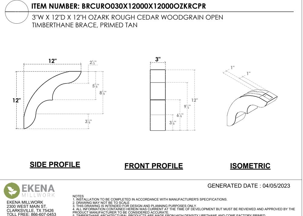
5. TIMBERTHANE ARCHITECTURAL PRODUCTS ARE MADE FROM HIGH DENSITY URETHANE AND COME FACTORY PRIMED
