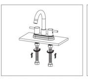
2. From the underside of counter top, install the hot and cold flexible supply lines to the faucet shanks tightening them securely.
