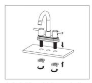
1. Install faucet into counter top, and tighten shank nuts down on the underside of the counter top with a basin wrench, ensuring the faucet is in the proper position.
