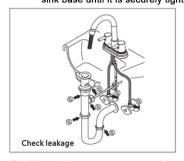
7. Close the pop up assembly and fill the sink to the overflow hole (if applicable) with water for at least 5 minutes to check the drain for leaks.
