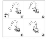
6. Remove the aerator from the spout and turn on hot and cold water to flush any air and debris in the water lines. Reattach the aerator.
