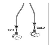
3. From the underside of the sink, Connect the open ends of the hot and cold supply lines to the shut off vales. Ensure the faucet is in the off position and turn on the shut off valves. Check for leaks on the supply line connections.
