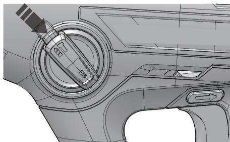
To change the operation mode, push the release button and turn the mode selection switch to the correct position until it clicks.
