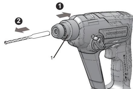
1. Pull back the clamp collar and remove the bit.
