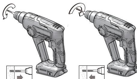
1. When the switch is on the left side of the switch trigger, the bit direction is forward (tightening).
