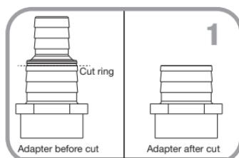
**Step 1.** If using the largest tubing size recommended for your pump, trim the tubing adapter using a hacksaw at the location indicated.
