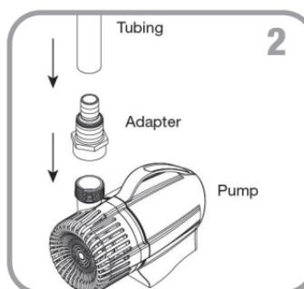
**Step 2.** Connect the adapter to the pump, and connect the tubing to the outlet of the adapter.
