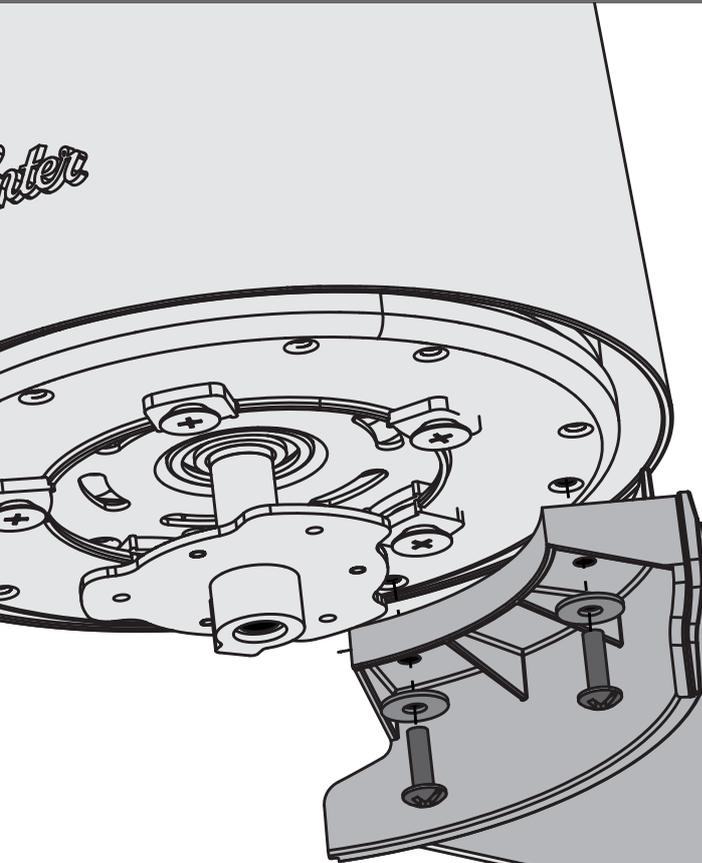
Put the blade washers found in the ■ hardware bag onto the blade screws found in the ▲ hardware bag. Then install the blade screws to secure each blade to the fan.
