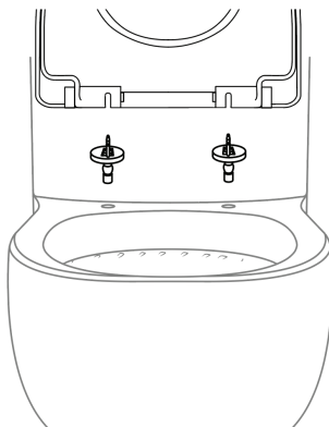
Install the hinges and seat Align the seat and bowl, then remove it
