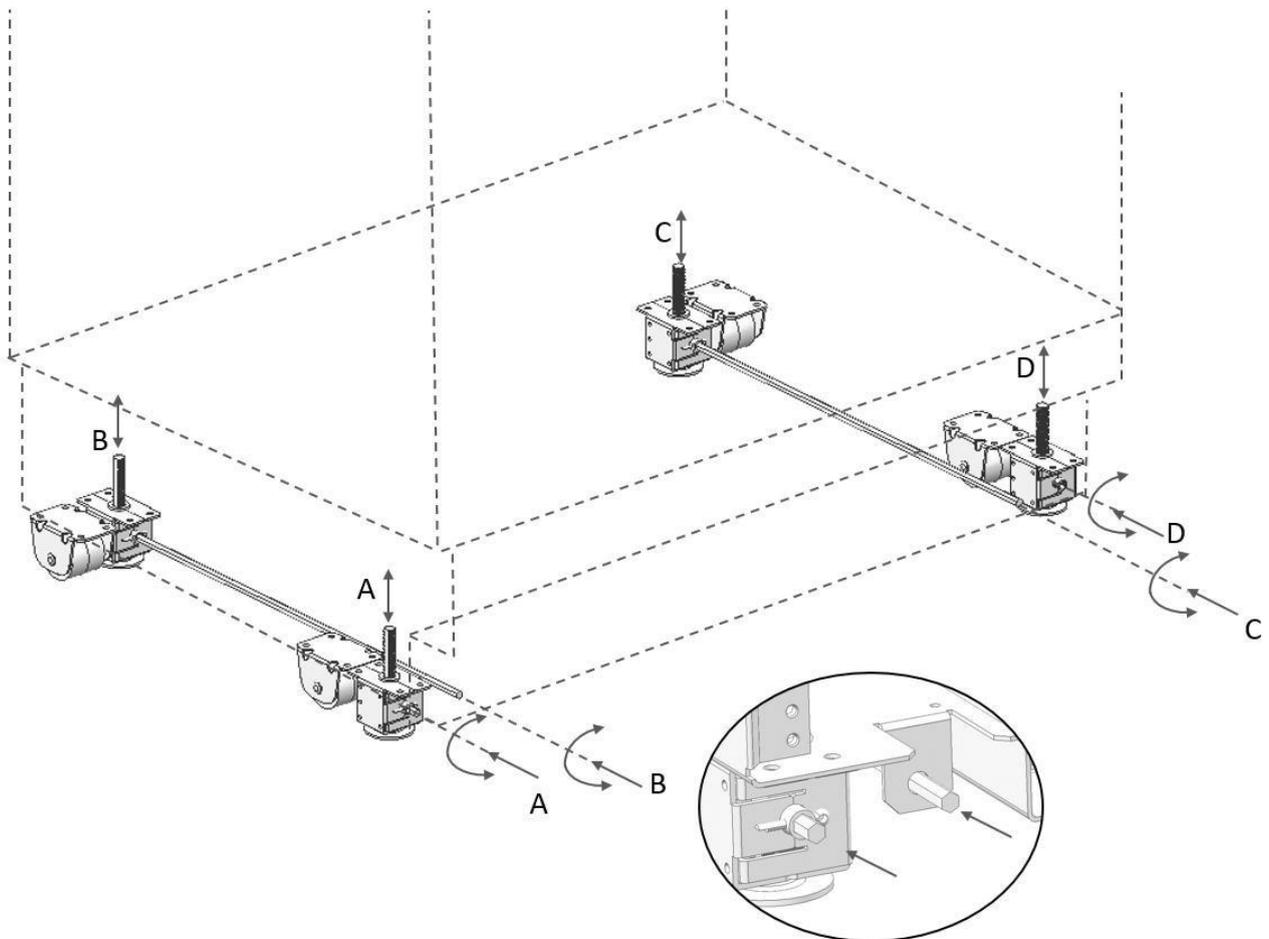
A/D –Turn the key clockwise to lift the front
