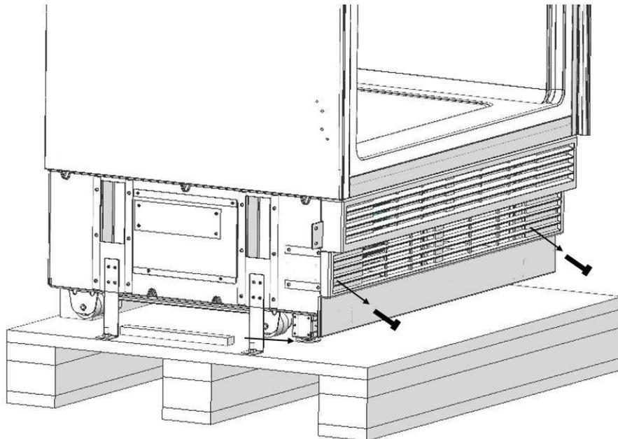
**Removing the Upper Vent Hole Part**
