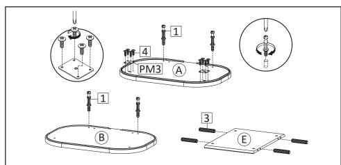
STEP1: Insert Cambolt (HW1) into Top Board (A) and Bottom Board (B). Insert Mounting Plate (HW PM3) secure with Screw M4.5x12.5mm (HW4) Into Top Board (A). Insert Dowel (HW3) into Back Board (E).
