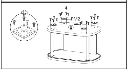
**STEP4**: Install Mounting Plate (HW PM2) Into Bottom Board (B). Secure with Screw M4.5x12.5mm (HW4) as figure.
