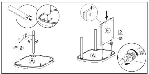
**STEP2**: Install Pillar (F) into Top Board (A). Tighten by rotating the Pillar clockwise. Attach Back Board (E), please notice the chamfer edge position as image. Insert Camlock (HW2) then tighten using screwdriver.
