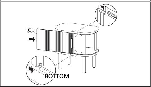
**STEP7**: Insert the Door (C) into the track. Carefully examine the tambour door. The side with plastic insert is placed at bottom track, while the side without plastic insert inside groove is for upper track.
