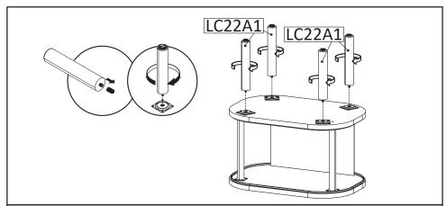
**STEP5**: Insert Leg (LC22A1) into Mounting Plate, tighten by rotating the leg clockwise.
