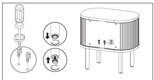
**STEP9**: Insert Stopper (HW8) into Bottom Board (B) position as the above image. Place your furniture on lever floor. The legs come with adjustable leveler, adjust it as needed until your furniture stands steadily on the floor.
