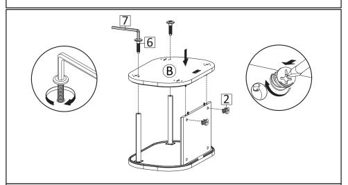
STEP3: Place Bottom Board (B) with the bolts of pillars get through the holes. Secure with Screw M6x30mm (HW6), tighten screws using Allen Key (HW7) as figure. Insert Camlock (HW2) then tighten using screwdriver.
