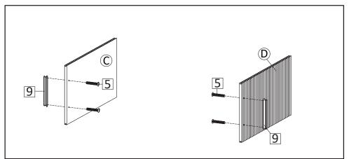
**STEP6**: Insert Handle (HW9) secure with Screw M4x16mm (HW5) into the holes on Doors (C&D).
