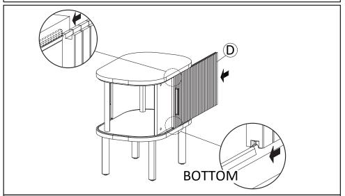
**STEP8**: Insert the Door (D) into the track. Carefully examine the tambour door. The side with plastic insert is placed at bottom track, while the side without plastic insert inside groove is for upper track.
