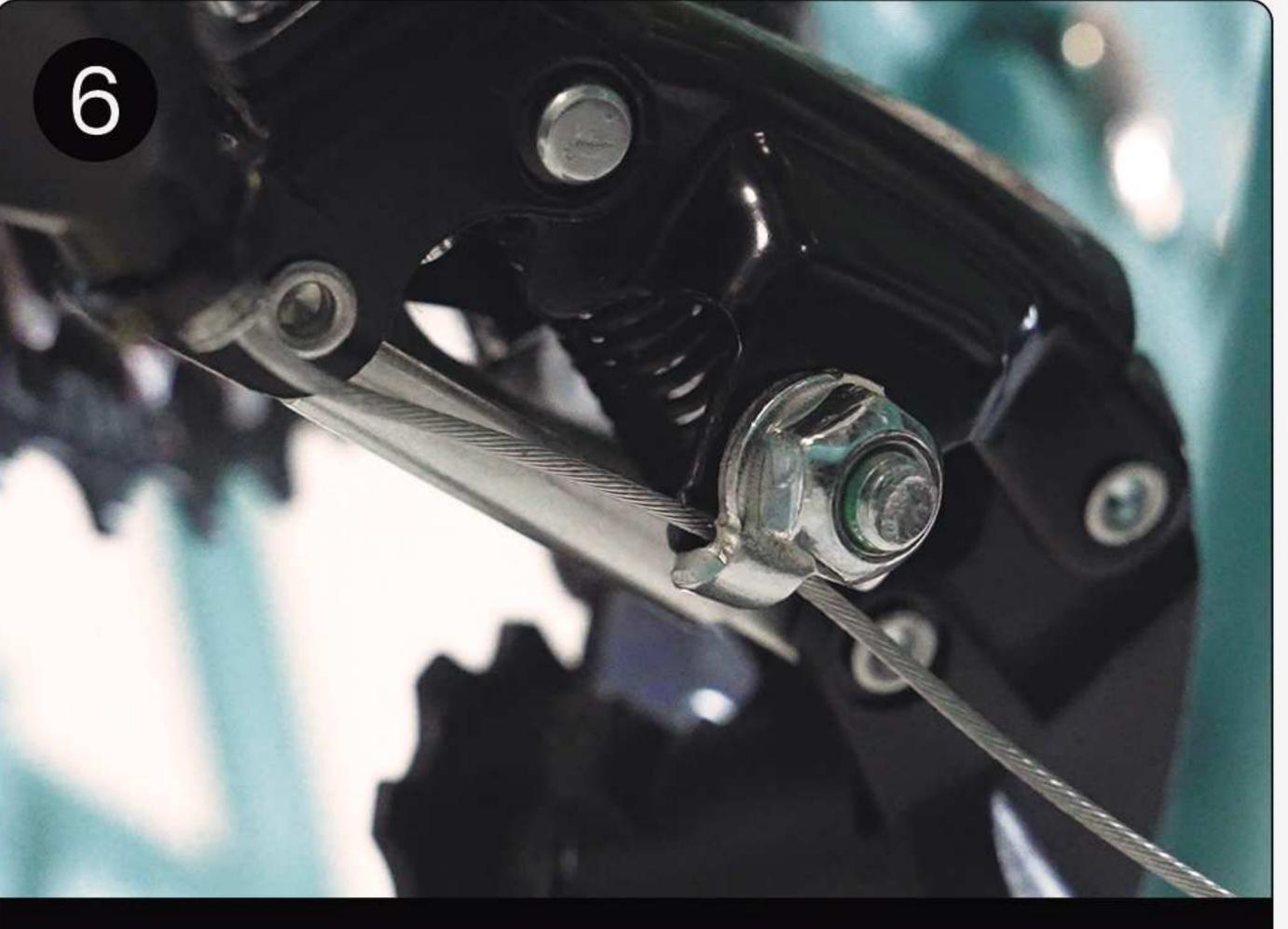
Check to ensure that screws retaining the brake cable on the derailleur are tightened.
