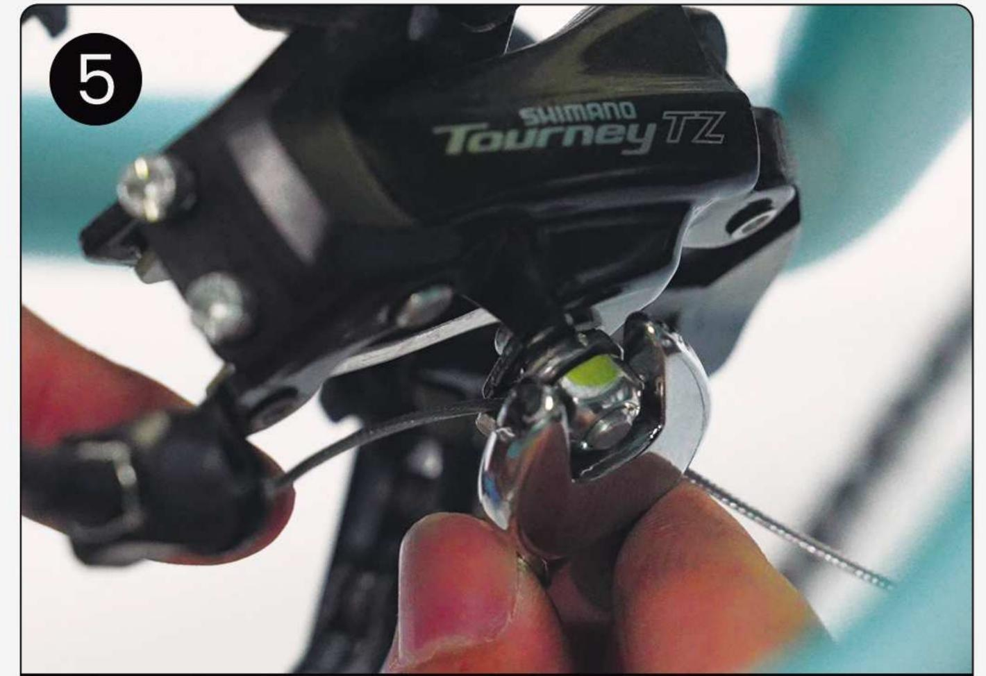
Loosen the cable retaining bolt as shown and thread the shift cable into position before tightening.
