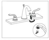
7. Remove the aerator from the spout and turn on hot and cold water to flush any air and debris in the water lines. Reattach the aerator.
