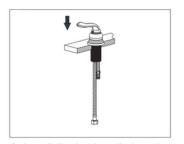
2. install the hot handle into the left side hole and the cold into the right side hole.
