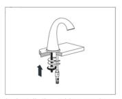
1. Install the rubber washer, metal washer and metal nut onto shank under countertop and hand tighten. Ensure the spout is in the proper position and tighten down firmly.
