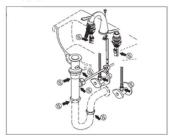
8. Close the pop up assembly and fill the sink to the overflow hole (if applicable) with water for at least 5 minutes to check the drain for leaks.
