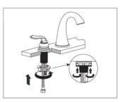
3.Install metal washer onto shank under countertop and hand tighten. Ensure the handles are in the proper position and tighten down firmly.
