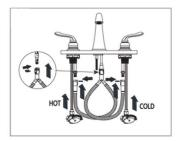
4. Connect the hot and cold supply lines to the shut off valves. Insert the trident fitting onto the spout shank adapter. Connect the hot and cold trident lines to the adapters on the bottom of the handles. Turn on shut off valves and check for leaks on the water supply lines.
