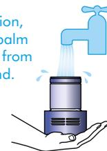
Filter with hand over the open end with arrows showing a shaking motion.
