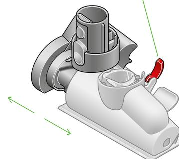
Remove any hair or fibres that have been wrapped around the brush bar.
