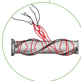
Remove any hair or fibres that have been wrapped around the brush bar.
