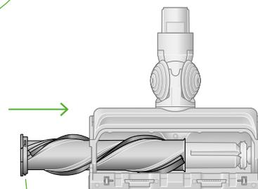
The removal of the brush bars showing the lock in a horizontal position and the unlock symbol at 90° anti-clockwise and lock symbol at 90° clockwise.
