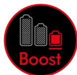
The screen showing the machine set to Boost mode with a red battery to show that this will give the shortest battery life of the three modes.
