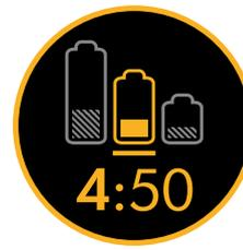
The screen with a battery time remaining shown as a number and as a half filled battery.
