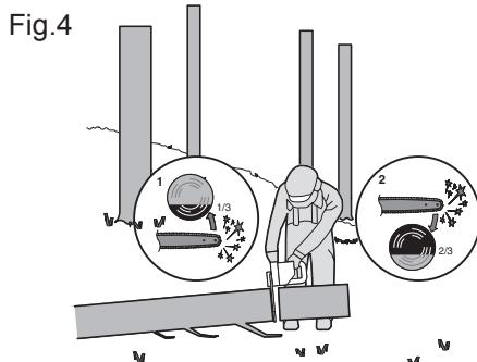
When the log is supported on both ends, as illustrated in Figure 5, cut 1/3 the diameter from the top (overbuck) (1). Then make the finished cut by underbucking (2) the lower 2/3 to meet the first cut.
