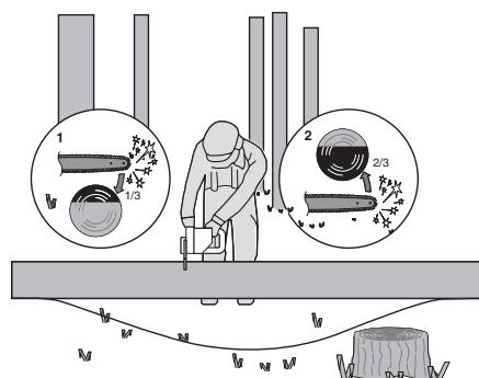
When bucking on a slope always stand on the uphill side of the log, as illustrated in Figure 6. When "cutting through", to maintain complete control release the cutting pressure near the end of the cut without relaxing your grip on the chain saw handles. Don't let the chain contact the ground. After completing the cut, wait for the saw chain to stop before you move the chain saw. Always stop the motor before moving from tree to tree.
