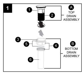
2. For the top drain assembly insert the top pop-up body (2) into the sink. Ensure that the top gasket (1) rests securely between the top of the sink and the top of the pop-up body (2) as shown in the Fig 2.
