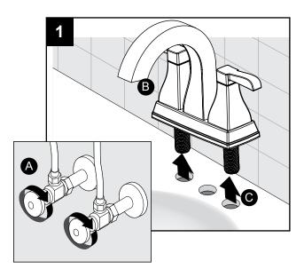
Ensure the gasket (B) is on the bottom of the new faucet (A). Place the faucet (A) through the mounting holes in the sink. Secure the faucet assembly (A) to the sink with the install nuts (C) and washers (D) provided. Screw the install nuts (C) and (D) washers to sink and hand-turn to tighten, as shown in the Fig 1.
