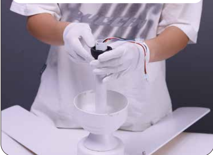
25. Put the hanger ball through the downrod
