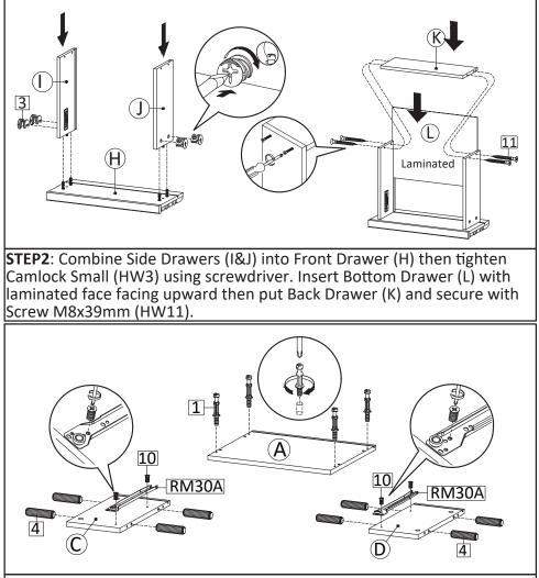
**STEP4**: Insert Cambolt Long (HW1) into Top Board (A). Insert Dowel Big (HW4) into Side Board Left (C) and Side Board Right (D). Continue with securing part of the Drawer Runner (HW RM30A) into position as the above image, using screw M6x10.5mm (HW10).
