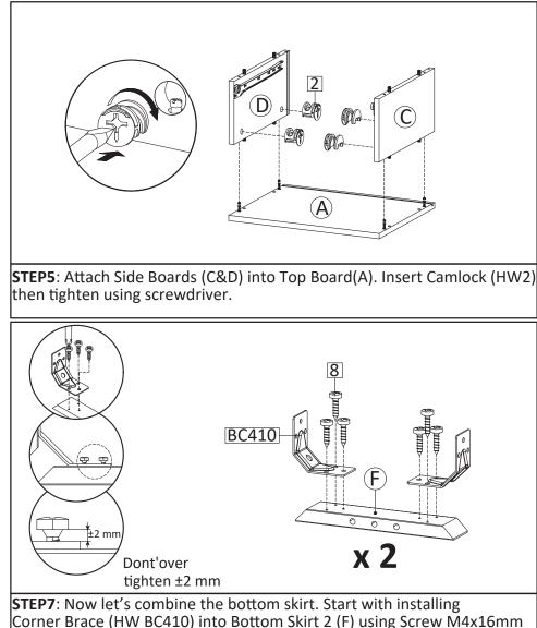
(HW8). Do not overtight screw yet, leave around 2mm gap.
