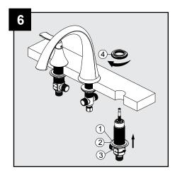
From underneath the deck, insert the valve body with the rubber washer (1), metal washer (2) and mounting nut (3) through hole on the right (cold) side. From above, thread the flange (4) onto valve body. Tighten the mounting nut (3), so that the flange (4) sits flush to the surface of working area. Then insert the other valve body through holes on the left (hot) side and install in the same way. Note: Hot side end valve is labeled.
