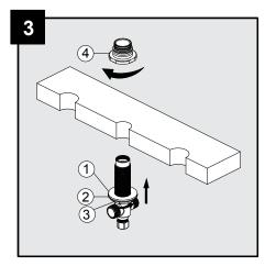
From underneath the deck, insert the middle body with the rubber washer (1), metal washer (2) and mounting nut (3) through hole. From above, thread the connector (4) onto middle body. Tighten the mounting nut (3), so that the connector (4) sits flush to the surface of working area. Note: The middle body must turn to the direction as shown in the diagram.
