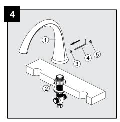
Place the spout assembly (1) onto the connector (2). Be sure the spout assembly (1) is resting firmly on the deck. Push down on spout assembly (1) and tighten set screw (3) with Allen wrench (Hex: 3.2mm, 4). Insert the cap (5).
