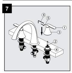
Place the handle assembly (1) onto the right (cold) valve (2). Then thread the handle seat (3) onto the flange (4). Place the set screw (5) into handle assembly (1) and tighten set screw (5) with Allen wrench (Hex: 2.5mm, 6), Place the other handle assembly onto the left (hot) valve and install the same way.
