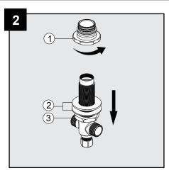
Remove connector (1) from the middle body. Adjust the washers (2) and mounting nut (3) to the bottom of middle body.
