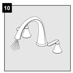
Turn on hot and cold water supplies and flush water lines for one minute. After flushing,turn the handles all the way off to shut off the water.
