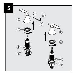
Unscrew the set screws (1) from the handle assemblies (2)with Allen wrench(Hex:2.5mm,6) and remove the handle assemblies (2) from the valve bodies. Loosen the flanges (3) from the valve bodies. Adjust the washers (4) and mounting nuts (5) to the bottom of valve bodies.
