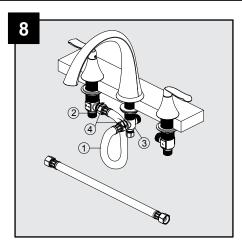
Connect the flexible water supply hose (1) to the bottom of valve bodies (2) as show. Align middle body (3) in a position which will allow maximum clearance to connect hoses. Carefully bend the hoses to fit available space. Carefully thread the hose couplings to the sides of the middle body (3). Tighten nut (4) securely with wrench.
