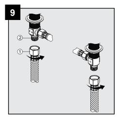
Connect a 1/2 in. IPS faucet connector (not included) to the water supplies underneath the sink using wrenches (not included).
