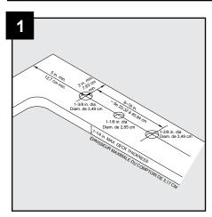
Drill holes in FINISHED DECK per diagram. NOTE: This kit is intended for installation up to 1-1/4 in. thick.
