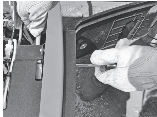
Figure 6-3. Inserting Power Wire (E1 or E2)
