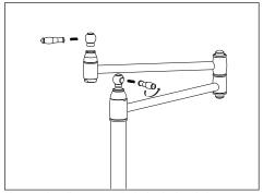
Unscrew handle counter clockwise by hand, then unscrew Screws using screwdrive, take out handle.
