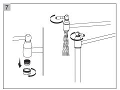
Remove the aerator and open both handles to flush debris from the faucet.
