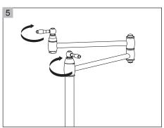
Turn both handles fully clockwise to the off position.
