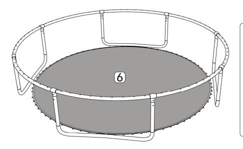
Lay out the Jumping Mat(#6)inside the frame on the floor as the picture on the left.
