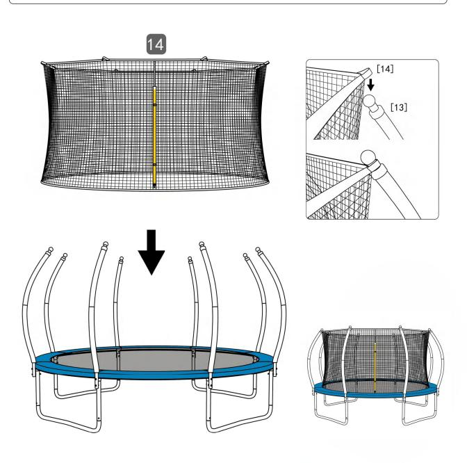
Components net ropes(#15), safety net(#14)through the bottom hole components, and parts cross around springs and fixed.
