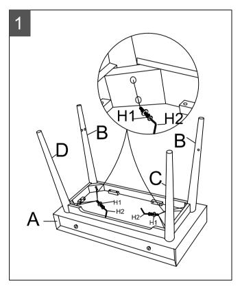
Step 1: Install facing left leg (C), facing right leg (D) and 2 legs (B) into cabinet with apron (A) as the shown picture. Put 8\*bolts (H1) right into holes and use Allen key (H2) to lock.
