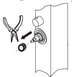
(5) Loosen the metal lock-ring and remove by tool (not available)
