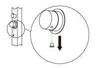
② Loosen the HEX screw with an allen wrench
