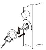
④ Press the button on the knob and put on the valve as shown ensuring the HEX screw points down
