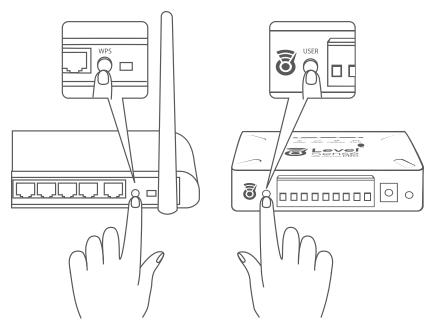
**TIP:** If the Cloud LED turns red following a WPS attempt, press the RESET button to restart the device. If the Cloud LED returns to red after restarting, check your router settings to see if WPS is enabled. Alternatively, try connecting with hotspot mode.
