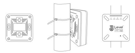
**TIP:** For larger diameter pipes, connect a second zip tie in series to extend the length of the zip tie.
