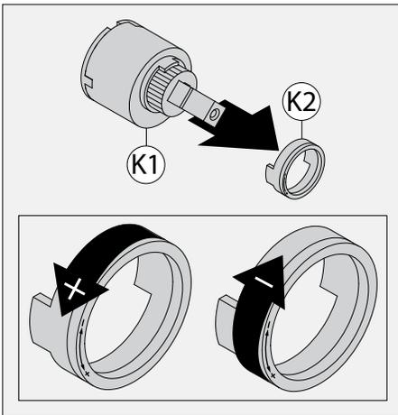
1) Remove limit stop (K2) from cartridge (K1). Turn limit stop counterclockwise to allow full handle turn to the hot position. Turn limit stop clockwise to limit handle turn to the hot position.
