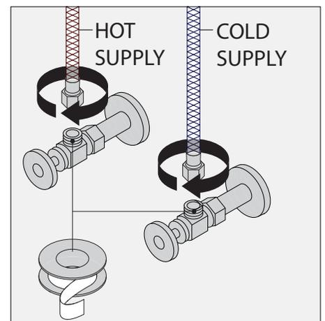
6) Connect hot supply hose (red stripe) and cold supply hose (blue stripe) to supply outlets.
