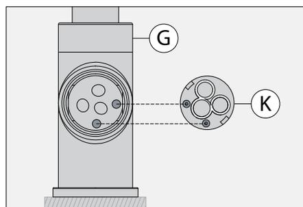
2) Inspect cartridge (K) for debris and replace cartridge if necessary. Align pegs on cartridge (K) with holes in faucet body (G) as shown above.
