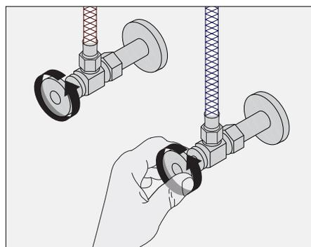
8) Turn on water supplies to flush lines.
