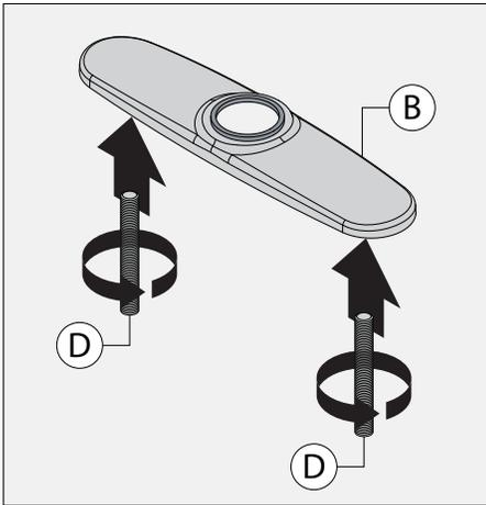
1) Thread studs (D) into deck plate (B).
