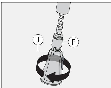
7) Remove spray wand (J) from pull-down hose coupling (F).
