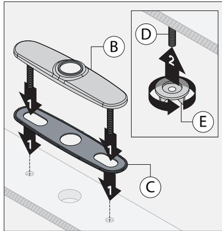
2) Install deck plate (B) and gasket (C) to deck surface. Thread mounting nuts (E) to studs (D) to secure deck plate (B) under deck.
