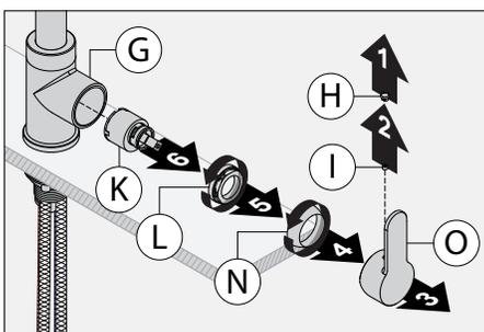
1) Remove plug button (H), set screw (I), collar (N), compression nut (L) and cartridge (K) from faucet body (G).
