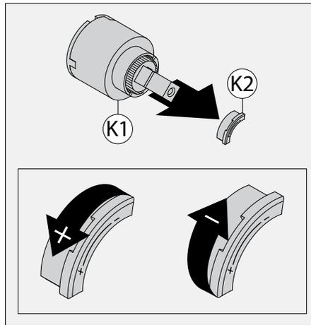
2) Remove limit stop (K2) from cartridge (K1). Turn limit stop counterclockwise to allow full handle turn to the hot position. Turn limit stop clockwise to limit handle turn to the hot position.
