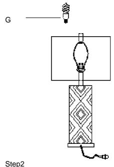
Insert the bulb(G) into the socket(C).
