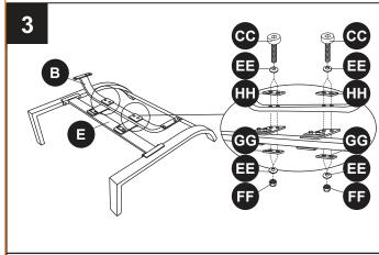
Hand tighten (CC). Once all bolts have been installed and hand tightened, go back and tighten firmly with wrench.
