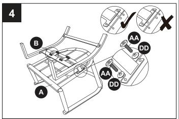
Hand tighten (AA). Once all bolts have been installed and hand tightened, go back and tighten firmly with wrench.
