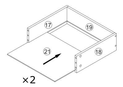
Insert bottom board 21 along grooves as shown. Insert bottom board 22 along grooves as shown.
