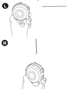
With the button pushed back to center, the laser line is projected vertically.
