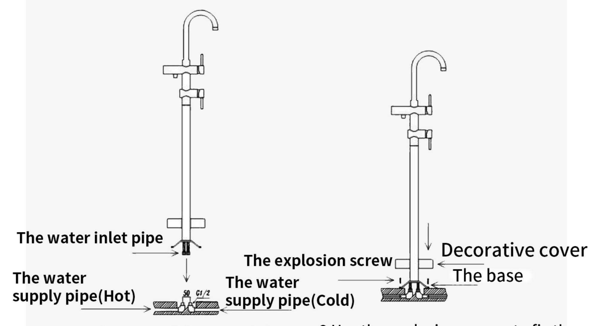
5.Connect another side of the water inlet pipe to the water supply pipe. Make sure they were screwed into the correct outlets for hot water and cold water.
