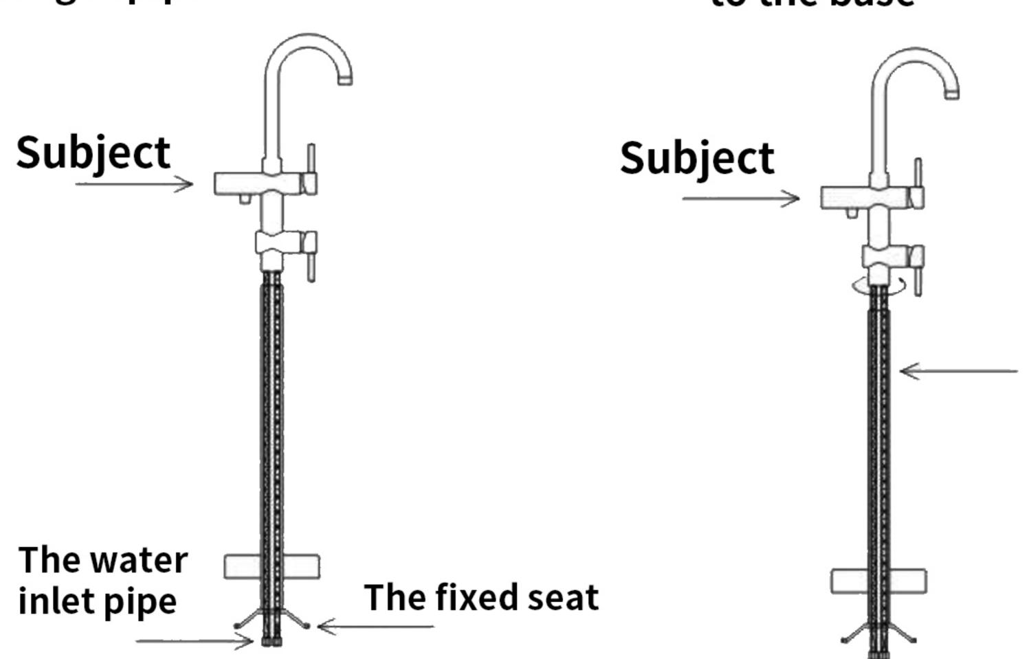
3.Screw and hand tighten the water inlet pipe to the water inelets of the subject (DO NOT USE SPANNER TO TIGHTEN AS IT CAN DAMAGF THE O-RING)Make sure the water inlet pipe were screwed into the correct inlets for hot water and cold water.
