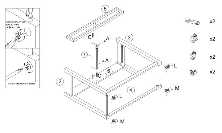
Step 4. Attach Front Frame (5) to Right & Left Side Frames (2 & 3) using Allen Bolts (F) as shown. Attach Towel Bar (K) to Right Side Frame (3) using Long Round Head Bolts (J) as shown. Now attach Top (1) using Cam Locks (A) & Wood Dowels (C) as shown.
