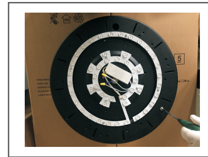
Step 4. Remove the main engine chassis screws.
