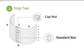
Cap nuts are used for top 2 rows, standard nuts are used for lower 4 rows. Assemble all corner panels: initially attach all bolts, washers and nuts loosely, and then tighten up using the wrench tool (as supplied) with a screwdriver/cordless drill.
