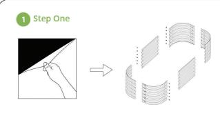
Remove protective films from both sides of panels, and lay panels on a flat surface according to the above configuration.
