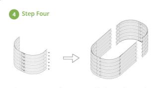
After corner panels are assembled, attach straight panels with corner panels using the same method. Make sure corner panels are attached outside of the straight panels.
