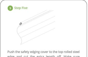
edge and cut the extra length off. Make sure edging is attached securely.
