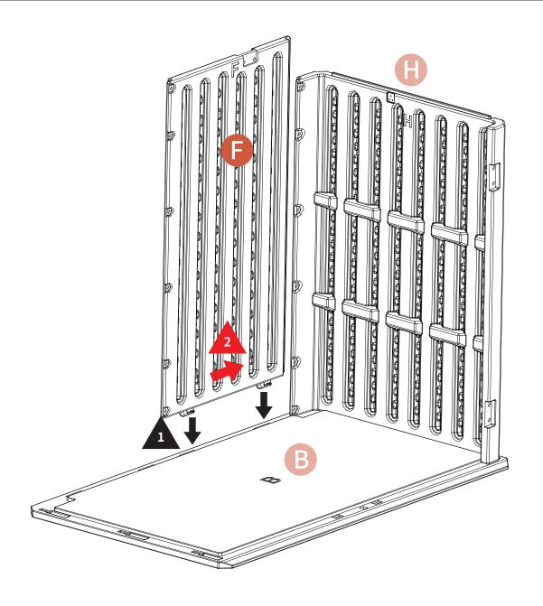
Insert parts F into part B's slots first, then make sure it can slide right to the full extent.
