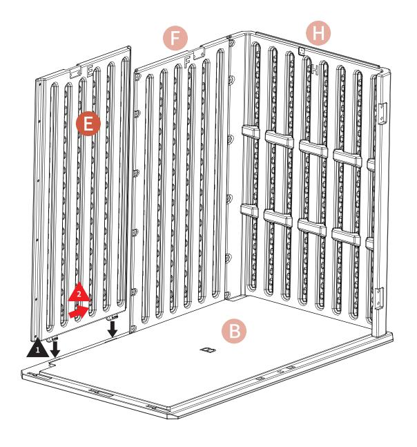
Insert parts E into part B's slots first, then make sure it can slide right to the full extent.
