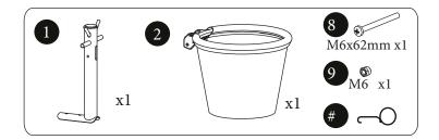
Use the parts to left for this step. Using the pictured tool, pull the spring of the basketball hoop(2) through large hole of the stand(1) and hook to the smaller hole below. Now attach the basketball hoop to the hoop stand using the M6x-62mm bolt and M6 nut.
