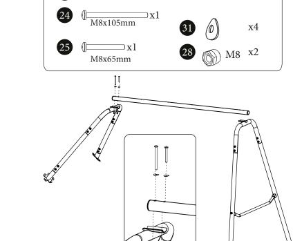
Using the parts pictured to the left, connect the top tube of the swing set(17) to the short A-frame piece that is connected to the geo dome.
