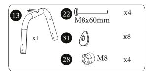
Using the parts pictured to the left, attach the "U" frame 1(13) to the poles from step 8 to complete the swing set A-frame.
