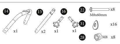
Using the parts pictured to the left connect the shorter A-frame pieces together.
