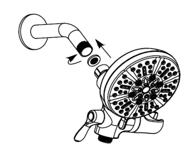
6. Attach 3 in 1 fixed mount shower head by threading clockwise onto shower arm with rotatable holder to the right and 3-way diverter control handle to the left. Use a wrench to tighten shower head nut to a snug fit. Do not over tighten. Wrap shower head nut with a cloth if you are using pliers.
