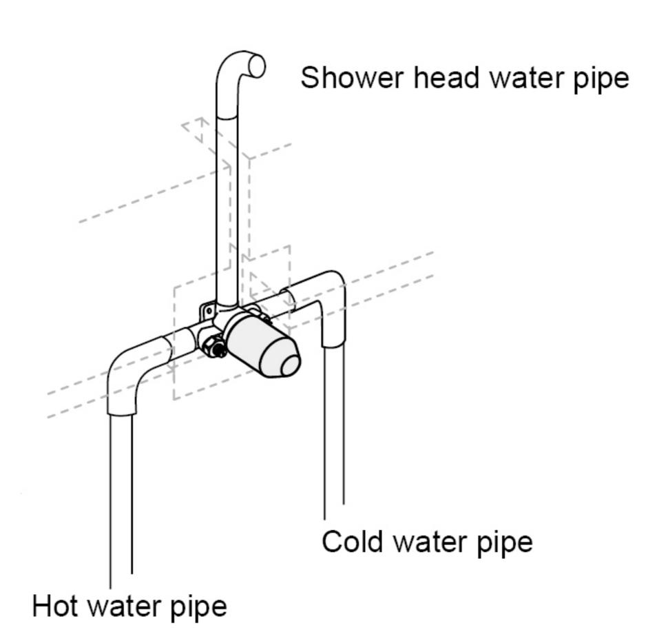
3. Connect water pipes to shower valve body as picture shows. And then install the shower valve body with screws.
