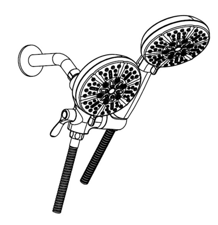
8. Place hand-held shower head in rotatable holder. Point all shower heads away from you and turn on the water full force. Check for leaks. Re-tighten all connectors if necessary.
