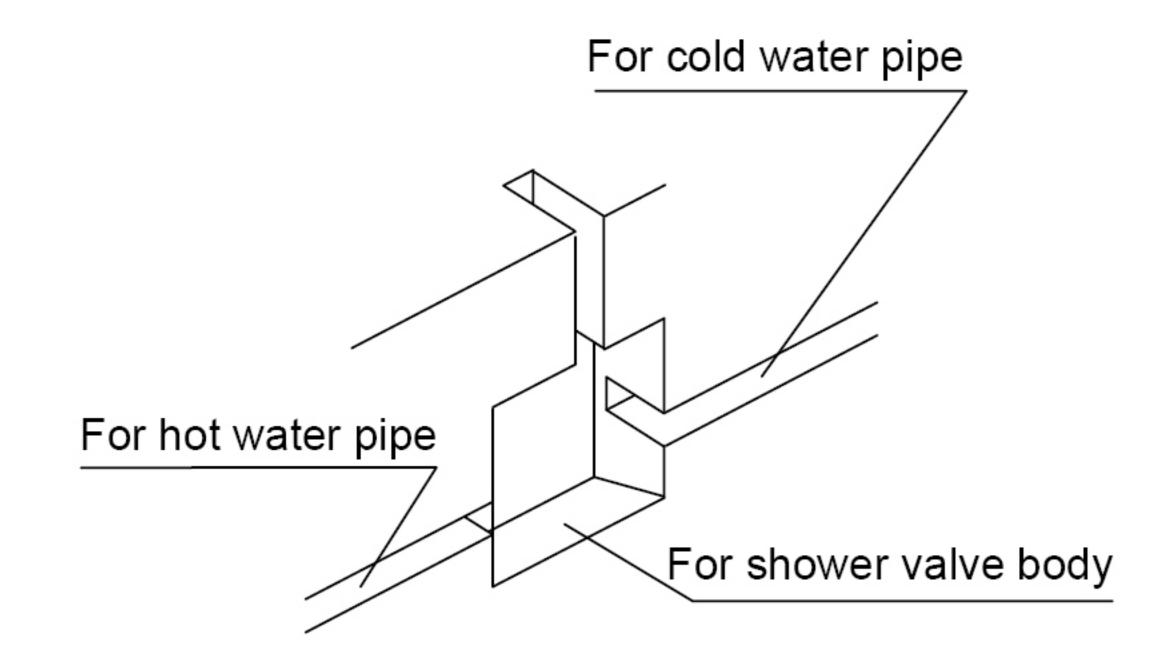
Use special tools to chisel holes on wall for installing, shower valve body and water pipe.
