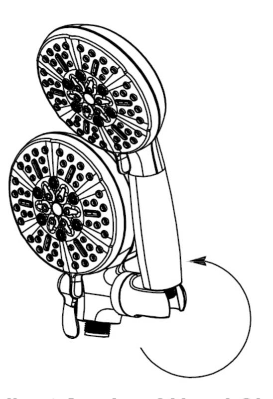
To Adjust Angle of Hand Shower Rotate holder in vertical direction to set desired hand shower angle.
