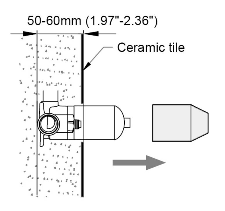
Switch on/off the cartridge, check all connectors without any leakage.
