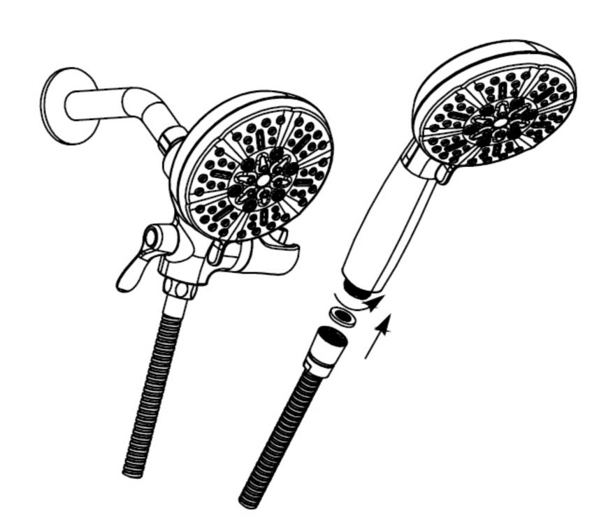
Locate the hose end with short hose nut and hand tighten to shower head.
