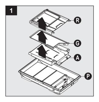
2. From left side of the saw, push water tray (P) into frame and stand assembly.
