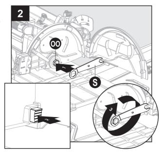
3. Remove arbor nut (OO) and outer washer (QQ), leaving inner washer on the arbor.
