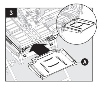
4. Place hook on the rear extension tray-2 (R) into the matching hole on rear extension tray-1 (A). Lower down to horizontal position.
