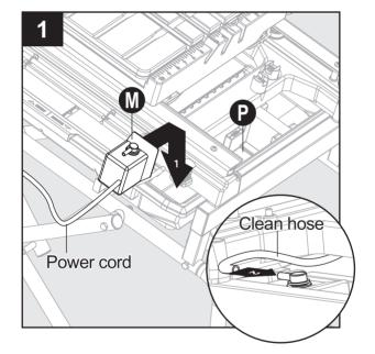
2. Pull the plug for pump out from the opening molded in the water tray. Push back rubber boot on the electrical cord and plug water pump into receptacle. Pull boot cover cord connections to help keep water off plug. Any excess cord can be wrapped on the two hooks.
