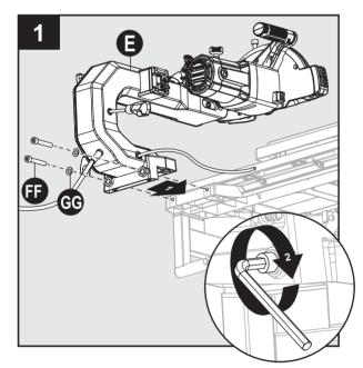
2. Insert hex cap screws (FF) through flat washers (GG) and into holes of motor head assembly (E) and top side of frame. Secure with hex wrench.
