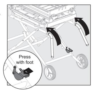
• Push the saw until the release lever clicks and locks into place.
