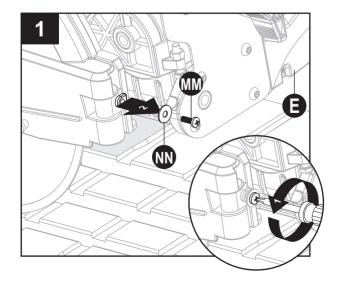
2. Attach the rear rubber flap (C) to the back of blade guard with big flat washer (NN) and screw (MM) (removed in previous step).
