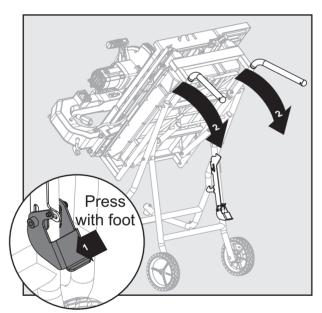
• With your hands on the handles, push the stand toward the ground until the saw is in an open position.
