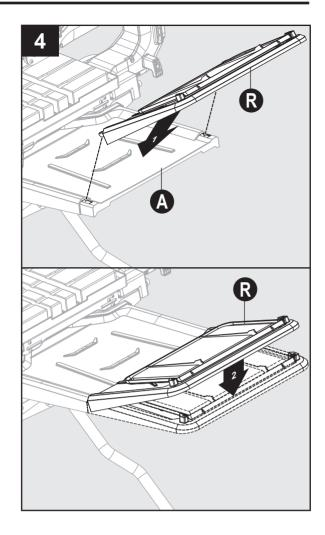
5. Rotate flap on rear extension tray-2 (R) to vertical position.
