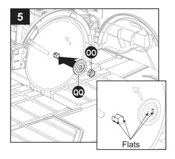
6. Using arbor wrench (S), press arbor lock (located on inside of motor head assembly) and tighten arbor nut (OO) securely.
