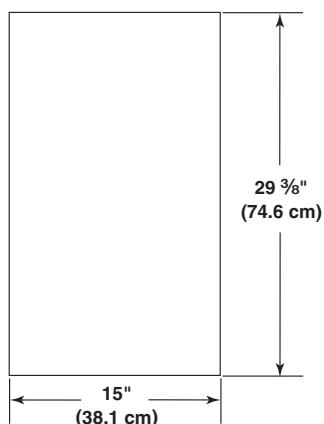
The panel should be a minimum of 1/2" (13 mm) thick.
