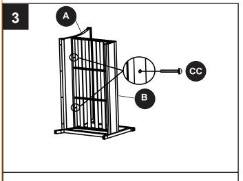
Hand tighten CC. Do not tighten until all bolts have been installed.
