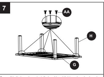
Once all bolts have been installed and hand tightened, go back and tighten firmly.
