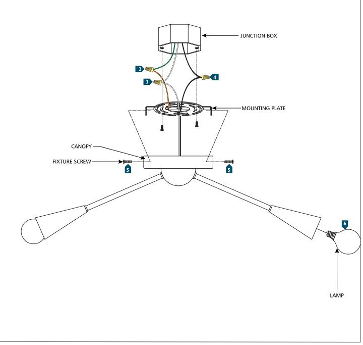
Secure the mounting plate to the junction box.
