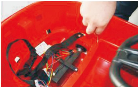
4:Seat installation: remove the screws on the body.
