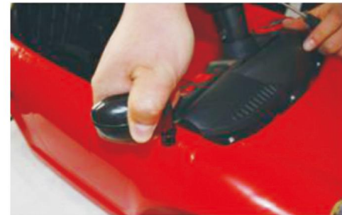
6:Install the reflector: install the reflector downwards on the car body and just hear the "click" sound.
