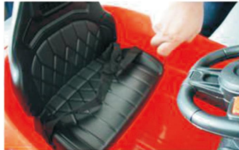
5:Seat installation: Place the seat on the body and tighten it with the removed screws.
