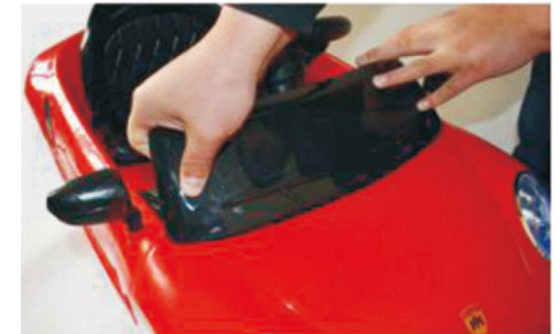
7:Install the front windshield: install the front windshield downwards on the body.
