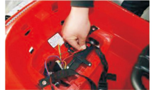
3:Install the power supply: Connect the power cord and connect the red terminal to the red connector.
