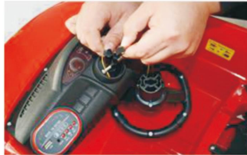
1:Music plug-in connection: connect the line before installing the steering wheel as shown in the figure.
