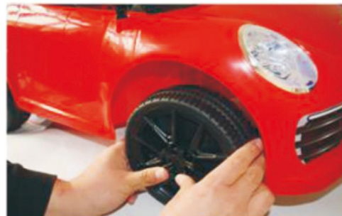
9:Fix the wheel with a split pin and cover the wheel cover.
