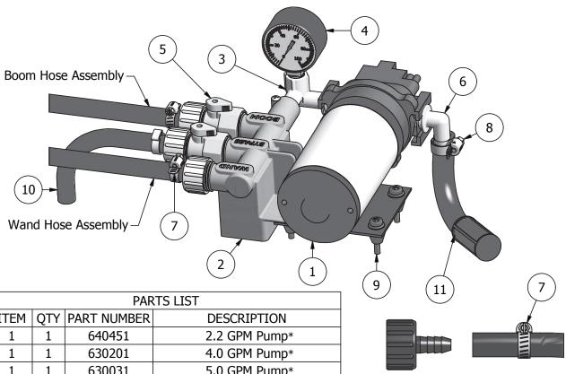
ITEM 1 1 630031 5.0 GPM Pump\* 2 1 600289 Manifold Body 3 1 600291 Elbow (2.2 pumps) 3 1 600292 Elbow (4.0 & 5.0 pumps) 4 600129 Gauge 0-100 PSI 1 5 2 600216 Inline Valve 600287 QD EL 12 6 1 7 2 600120 5/8" Hose Clamp 8 1 600288 1/2" Hose Clamp 9 4 600130 10-24 x 1.25 Screw 10 1 600213 Relief Hose Assembly 3 11 600315 Suction Hose Assembly 12 1 600298 Cap Assembly (not shown)
