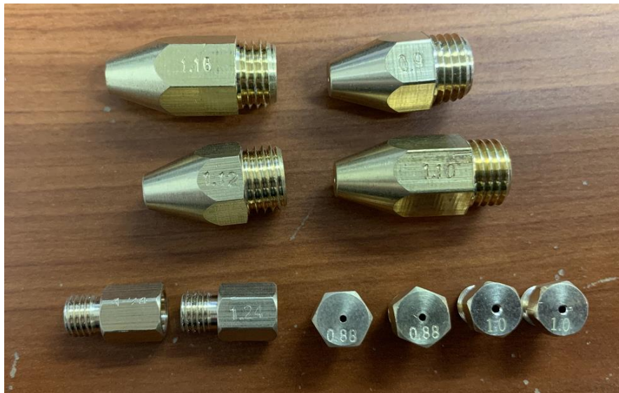
Top: (Left to right) Griddle Orifice, Large Oven Broil Burner Orifice Middle: (left to right) Large Oven Bake Burner Orifice, Small Oven Bake Burner Orifice Bottom: 4000BTU/6000BTU/8000BTU/9000BTU/18000BTU Top Burner Orifice
