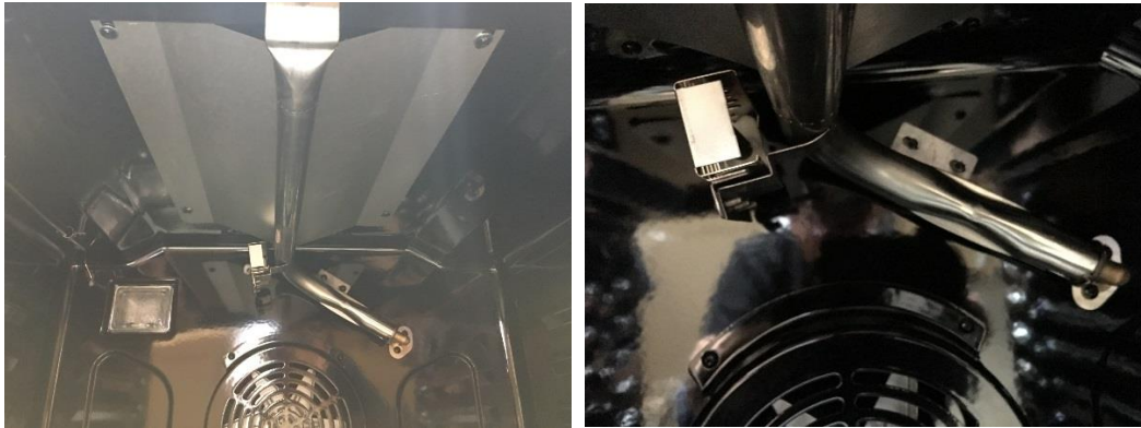
a. Broiler Burner is connected to Flame Tamer; b. Two screws on the back holding the burner to back oven panel;
