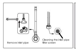
Cleaning and maintenance: Waterfall type: if the water flow weakens slightly after long-term use, the filter screen of the inlet pipe can be cleaned to change this phenomenon. (the filter screen of the water inlet pipe can filter large particle impurities in the water)
