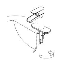
1.Make sure there is a Ø30-Ø33 Hole on the basin before fix the mixer, Unscrew the fitting ASSY from the bottom of the body, then get the body through the hole, don't forget to fix the o-ring between the bottom of the body and the basin.
