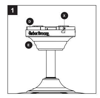
Secure the canopy (E) with the mounting bracket screws (X) previously removed (Step 4, page 8).
