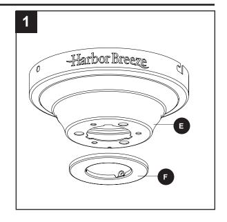
2. Remove three Phillips-head closemount screws (M) from the top of the motor assembly (N). Align the canopy (E) with the holes in the top of the motor assembly (N), then re-install the Phillips-head closemount screws (M) to secure the canopy (E) to the top of the motor assembly (N).
